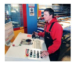
National Lumber runs automated saws guided by the SAPPHIRE BIM models, which are in turn driven by SAPPHIRE design files. As a result, National Lumber's components and framing kits are accurate to 1/16th inch.
