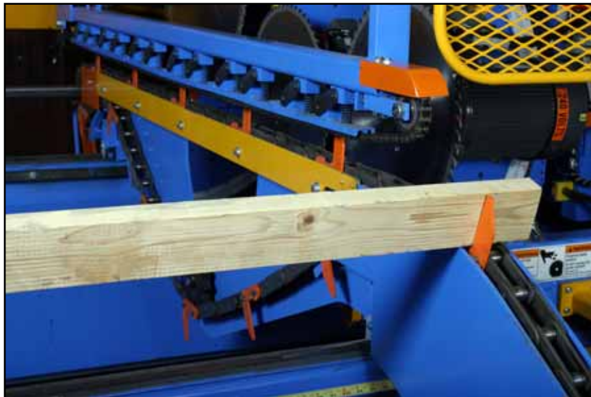
Figure 3-16: Infeed Conveyor Carrying Lumber in 2x4 Orientation
