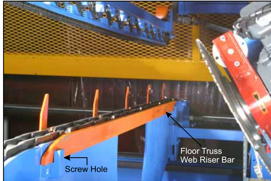
Figure 3-13: Attaching the Floor Truss Web Riser Bars
