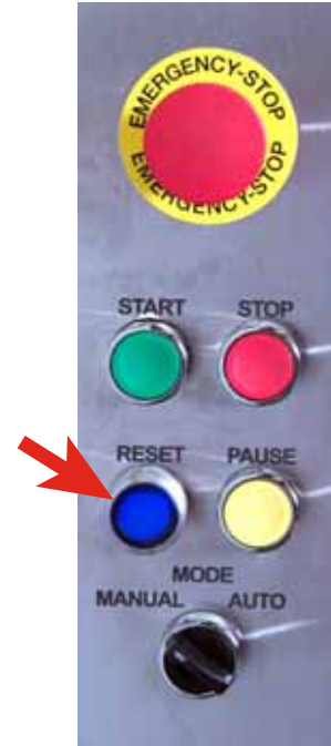
Figure 4-5: Reset Button on Operator Interface Panel
