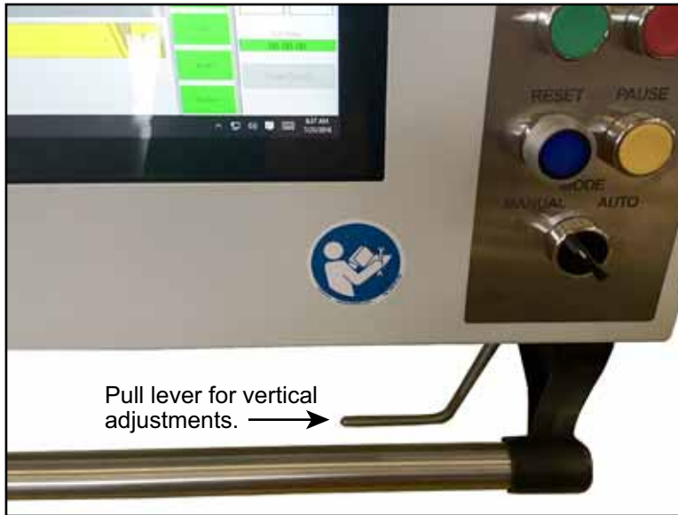
Figure 4-15: Moving the Touch Screen Up and Down
