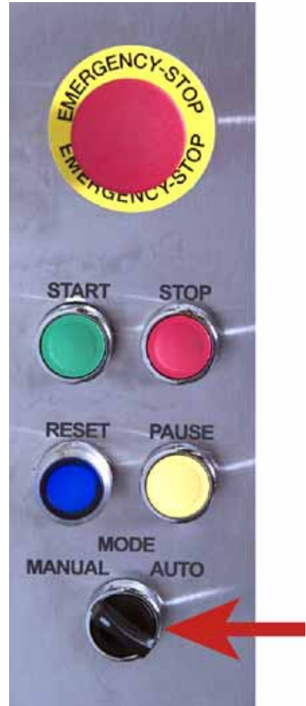
Figure 4-30: Mode Selector Switch Shown in Manual Mode
