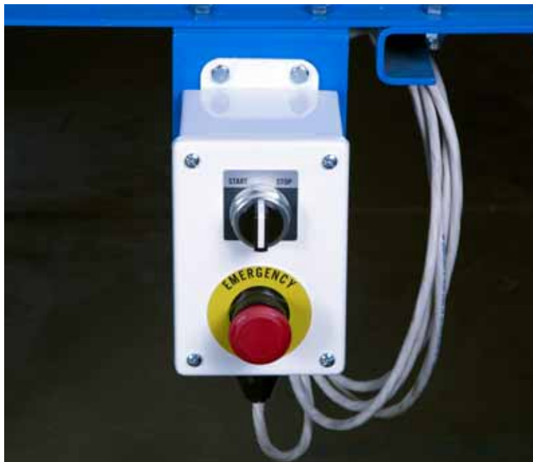
Figure 4-41: Control Station for Powered Skewed Conveyor
