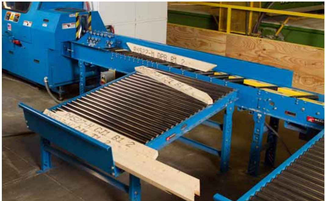
Figure 2-4: Optional Powered Skewed Conveyor Attached to Saw
